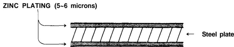
1. Before spot welding the zinc-plated steel plate, remove the paint from both sides of the flange to be welded. Apply sealer to the flange after welding.
