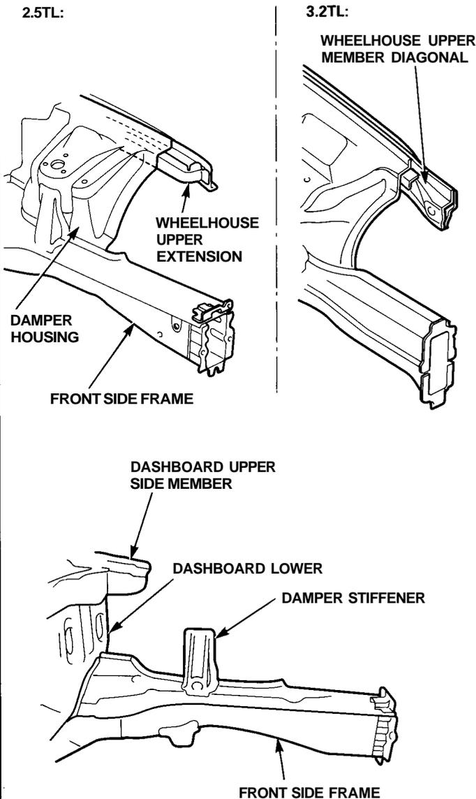
6. Set the new front wheelhouse and damper housing.
