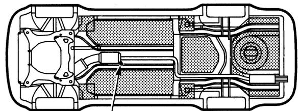
**SECONDARY HEATED OXYGEN SENSOR**
