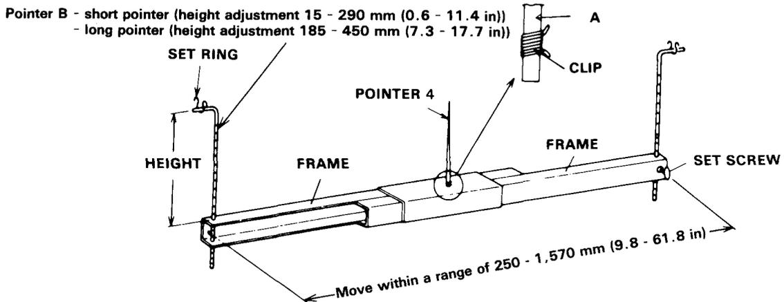
When measuring body dimensions, use a universal tram gauge.
